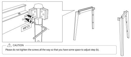
b. Plug the leg connector into the table fixture as shown below, and install the bridge connector to the base frame.
